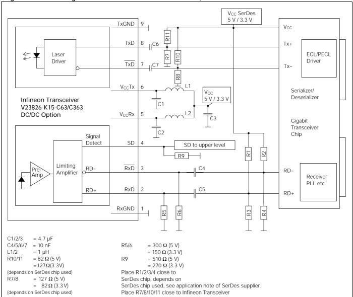
Values of R1/2/3/4 may vary as long as proper 50  $\Omega$  termination to V $_{EE}$  or 100  $\Omega$  differential is provided. The power supply filtering is required for good EMI performance. Use short tracks from the inductor L1/L2 to the module V $_{CC}$ RX/V $_{CC}$ TX. We recommend a GND plane under the module for getting good EMI performance.
